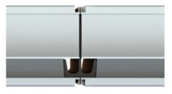
Push the windows together aligning the mullion with the j-channel pockets.
