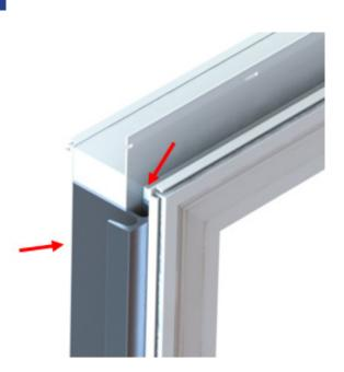
Apply the mullion to the side of the window aligning the mullion with the j-channel pocket. Make sure the mullion doesn't stick pass the j-channel pocket. Press firmly to engage the double-sided tape.
