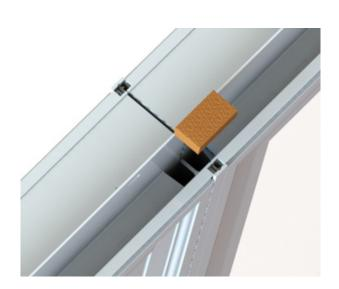
Install the mull key flush with one side of unit and hammer into place with rubber hammer.
