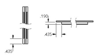
Cut the C-mull keys to the length of the unit (width or height) to be mulled. Notch both ends of mull key with a utility knife or chisel per dimension shown above.
